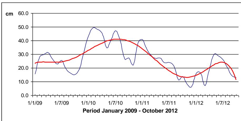
**Fig. 5 - Sea level oscillations recorded by the Constanța maregraph during January 2009 - October 2012 (monthly means)**
