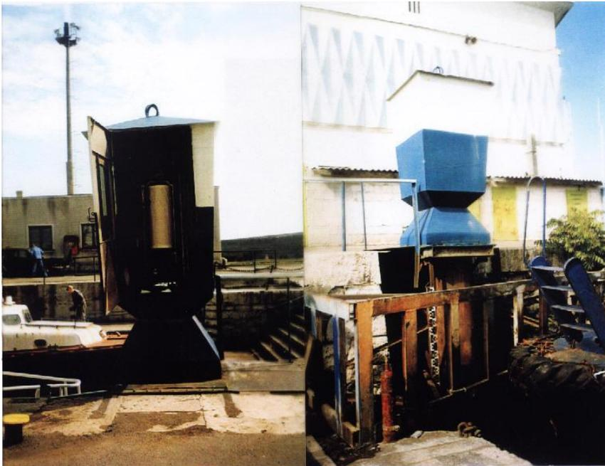
**Photo 1 - The maregraph in the Constanța Harbor and the hydrometer**
