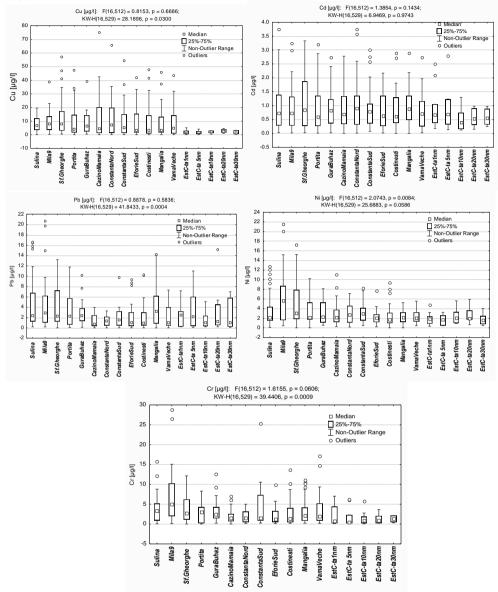
Fig. 2 - Spatial distribution of heavy metal concentrations in seawater along profiles monitored during 2006-2011
