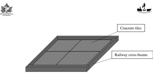
Fig. 2 - Concrete tile platforms
