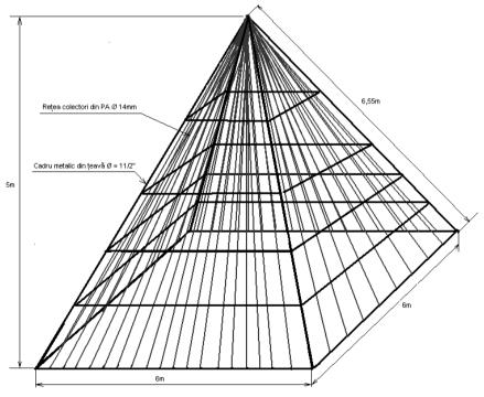
Fig. 4 - Submerged pyramid-shaped structure
