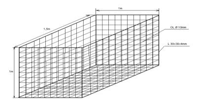
Fig. 3 - Metal frame for gabions
