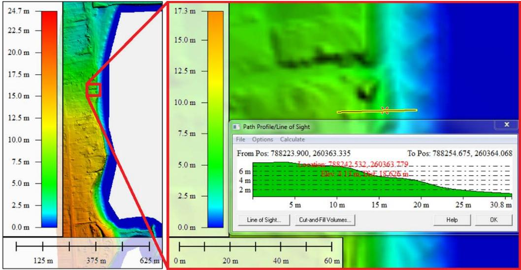
**Fig. 10.** Area of interest represented on the Digital Terrain Model (DTM) for 2 Mai, and (b) Cross-section of the cliff slope
