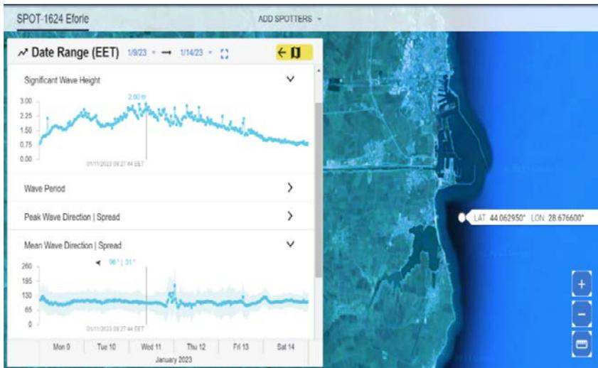
**Fig. 5.** Wave data recorded at Eforie station (significant wave height 2.60m, Wednesday 11.01.2023)
