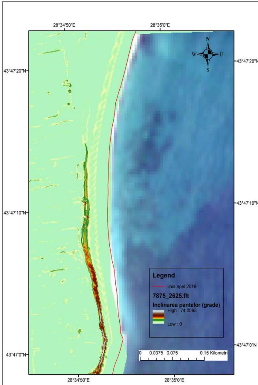
**Fig. 9.** Slope map (in degrees), derived from digital terrain model (DTM/2011), ArcGIS representation (coordinate system: Stereo 70)
