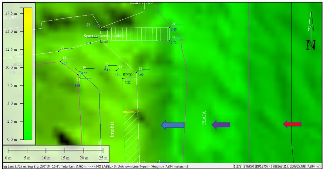
**Fig. 11.** Detail of the main components of the cliff-side shoreline in the 2 Mai area: in yellow, the distance of 3.7m from the crest of the cliff-side to the wall of the existing building on the cliff (red arrow – swash line, purple arrow - the cliff's foot, bleu arrow - the cliff's apex)
