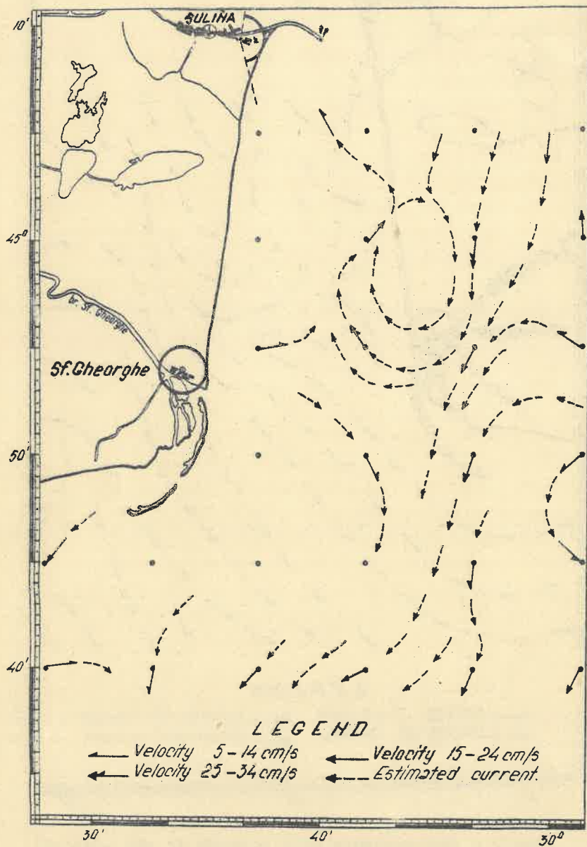
Fig.8 - Sea currents at 10 m depth in the zone of the Danube mouths (September 7-8, 1977).
