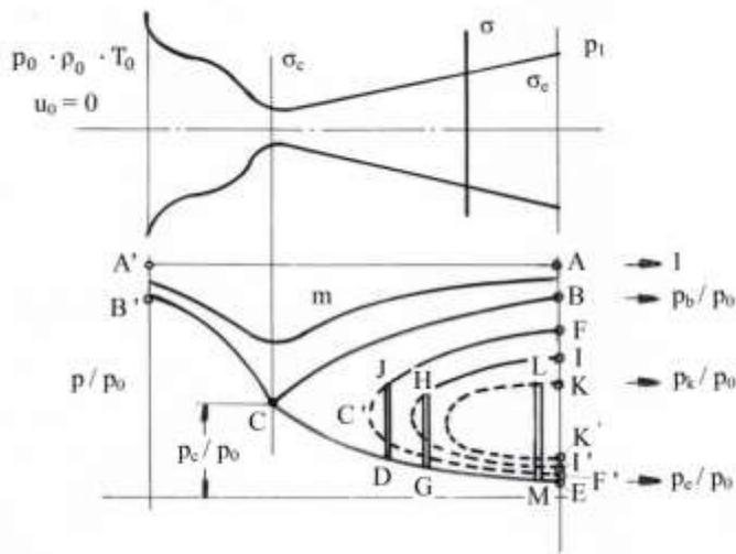
**Fig. 4.** Pressure distribution through the Laval nozzle.
