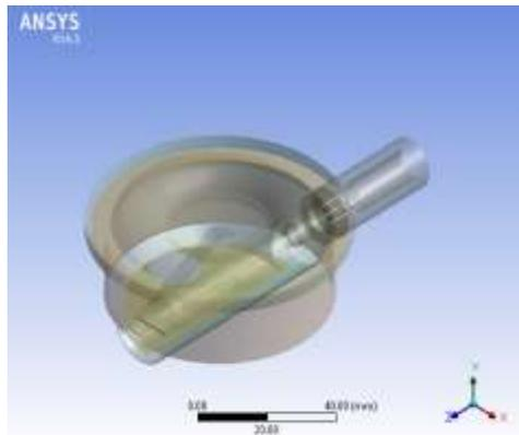
**Fig. 10.** Low pressure chamber of second stage Super Physalie.
