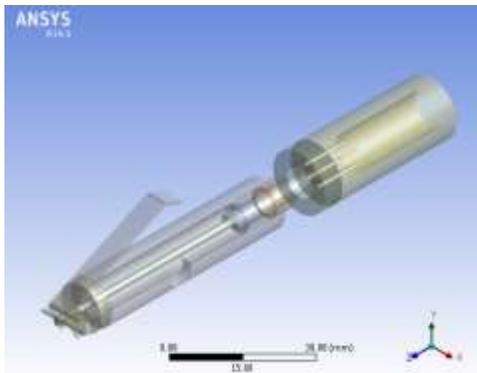
**Fig. 11** Intake mechanism of variant 1 Super Physalie.
