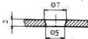
**Fig. 9.** Conical piston hole section variant 3.
