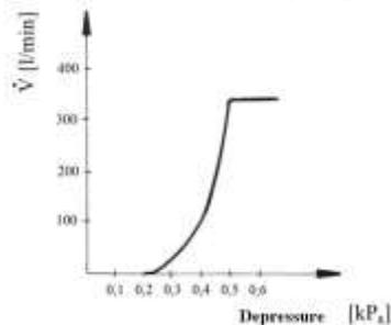
**Fig. 3.** Functional characteristic of the regulator in normobaric pressure.
