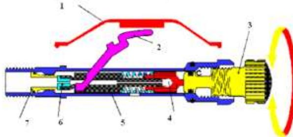
**Fig. 1.** Operating of a second stage regulator with cracking resistance control.
