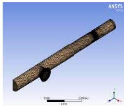
**Fig. 16.** The air circuit mesh in the intake mechanism for variant 3.
