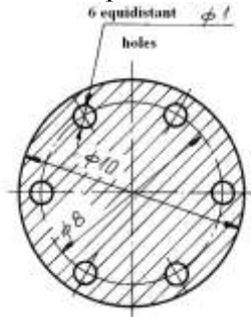
**Fig. 6.** Intake seat section variant 1.
