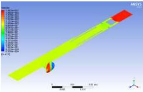
**Fig. 21.** Distributions of speed in a plane parallel to pl xz and to the air outlet, variant 2.
