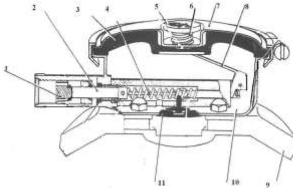
**Fig. 5.** Super Physalie regulator with downstream opening
