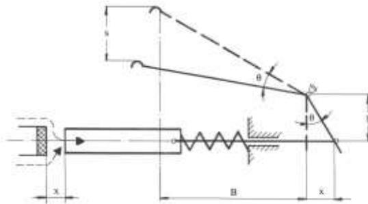
**Fig. 2.** Intake mechanism of the second stage regulator Super Physalie.
