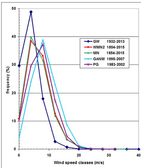
**Fig. 11. Long-term wind speed distributions on shore and offshore**
