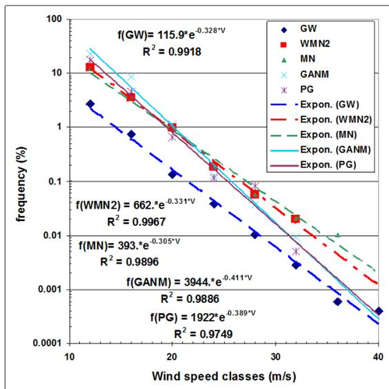
**Fig. 12. Long-term wind speed and distributions on shore and offshore (tails)**
