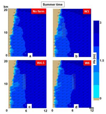
Fig. 2. The expected impact of the wind farm on the wave fields reported for the summer time, where: a) no farm; b) W3 scenario; c) W4.5 scenario and d) W6 scenario
