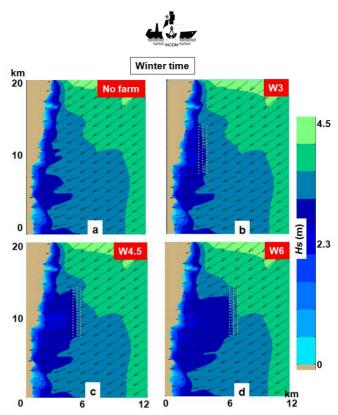
Fig. 4. The expected impact of the wind farm on the wave fields reported for the winter time, where: a) no farm; b) W3 scenario; c) W4.5 scenario and d) W6 scenario
