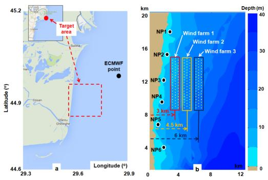
Fig. 1. Definition of the target area and set-up, where: a) overview of the target area; b) SWAN computational domain where can be observed the three case studies taken into account and also the locations of the reference points NP1-NP6
