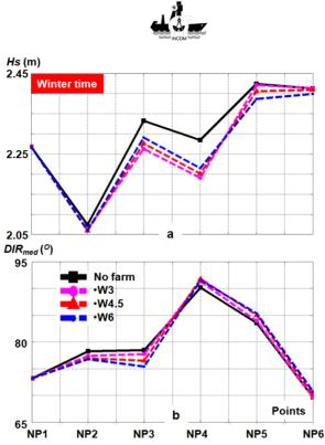
Fig. 5. The influence of the offshore wind farms during the winter time, reported for: a) *Hs* (m) parameter; *Dir* (°) parameter
