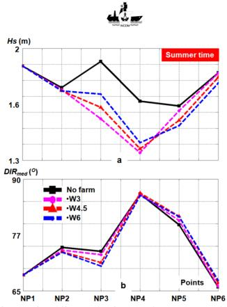
Fig. 3. The influence of the offshore wind farms during the summer time, reported for: a) Hs (m) parameter; Dir (°) parameter
