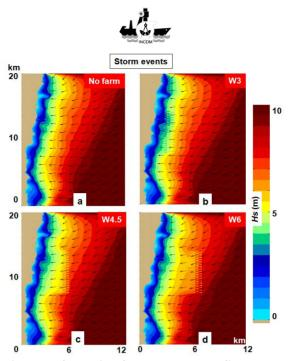
Fig. 6. The expected impact of the wind farm on the wave fields reported during a storm event, where: a) no farm; b) W3 scenario; c) W4.5 scenario and d) W6 scenario
