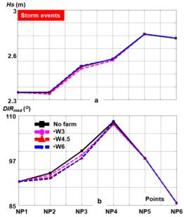
Fig. 7. The influence of the offshore wind farms during a storm event, reported for: a) *Hs* (m) parameter; *Dir* (°) parameter
